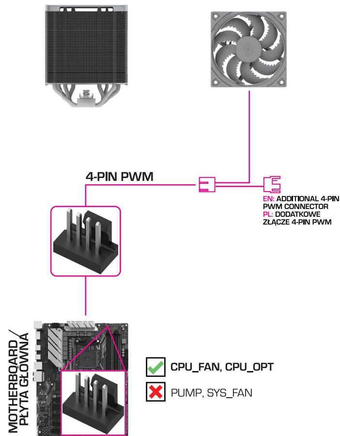
! EN: The pink line shows the connection required for automatic control of the Fera 5 fans' speed via motherboard. Connect the individual elements according to the pink diagram.
