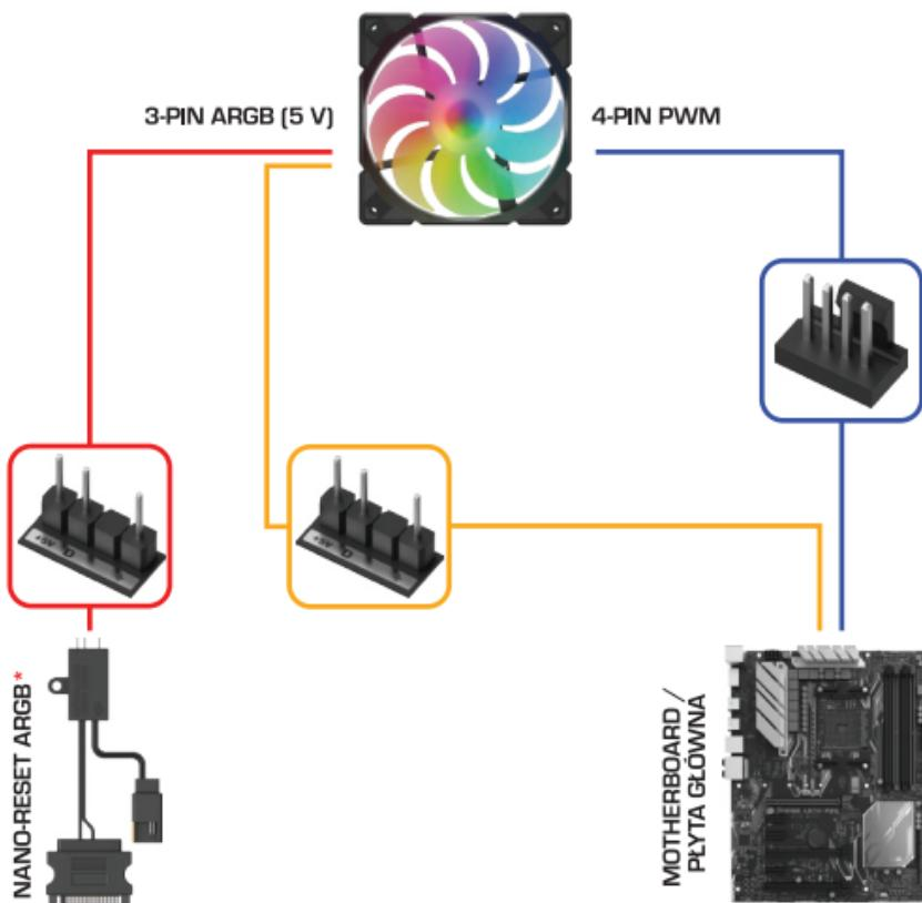
**A** EN: Choose A if you have a motherboard with 3-pin ARGB socket and want to control the ARGB lighting using the software from your motherboard manufacturer. If you chose B (control via motherboard), connect the individual elements according to the yellow lines only.
