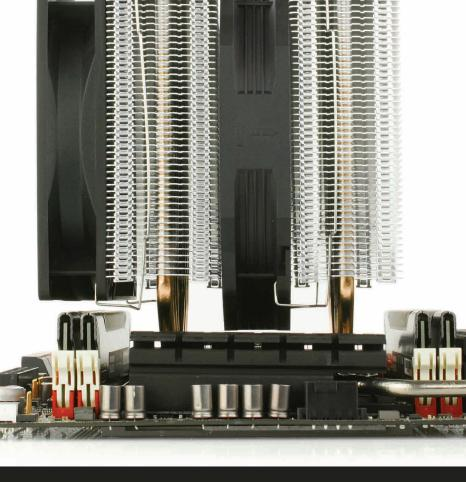
Grandis 2 XE1436 is the pinnacle of SilentiumPC CPU cooler lineup. This dual-radiator monster offers stellar cooling potential for the hottest processors on the market. The performance comes from massive heat dissipation area and the XE Technology, an additional solid copper heat spreader that transmits the heat from the CPU more efficiently to all six Φ6mm U-shaped heat-pipes unleashing their full potential.
